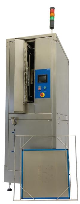
Specially designed to provide high cleaning performance, the stencil is introduced into the loading cell of the equipment and automatically immersed in the upright position and submitted to the superior cleaning performance of perpendicular ultrasound and is perfectly cleaned in just a few minutes. Alternatively, a spray under immersion system can replace the ultrasonic for the cleaning of your sensitive screens or stencils.
